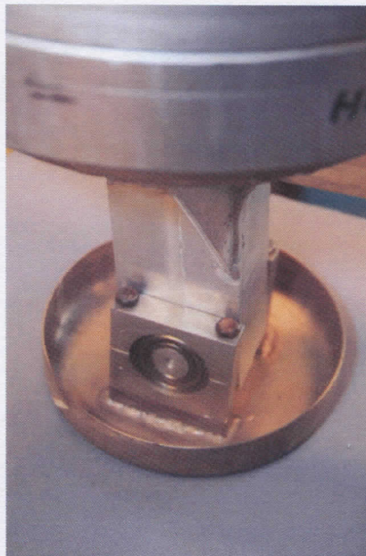
Fig 4: Static loading test of the seat
