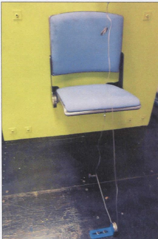
Fig.7. and 8: Test of tipping mechanism of the chair
