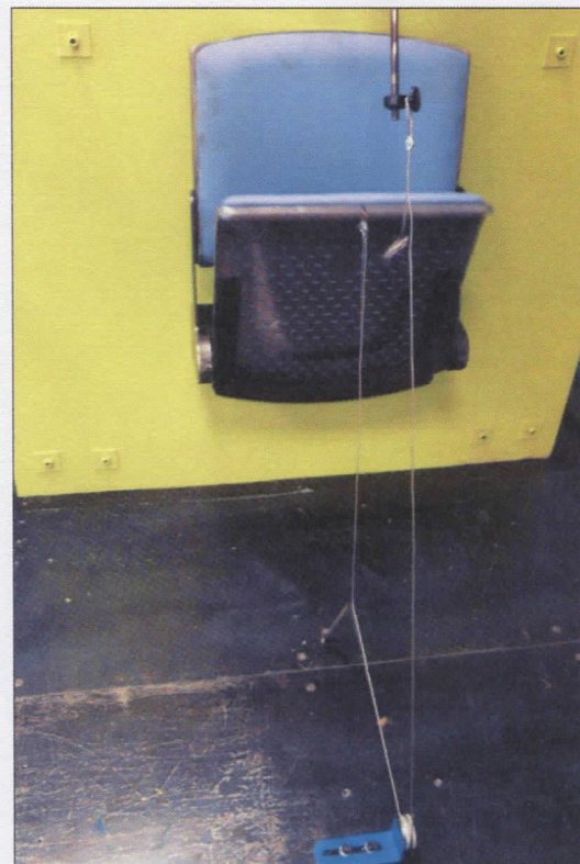
Fig.7. and 8: Test of tipping mechanism of the chair
